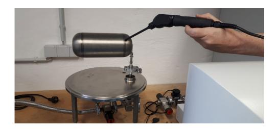
The sniffing test is one of the overpressure methods. The test sample is pressurised with helium via a test connection so that an overpressure is present. The sniffer probe which is connected to a leak detector can detect the helium escaping from a leak.
