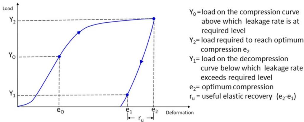
Fig.2: Characteristic curve of a Helicoflex seal for illustration of useful elastic recovery (according to [www.Techneticsgroup.com](http://www.Techneticsgroup.com))
