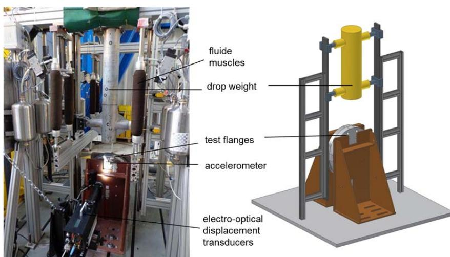
Fig.1: Test assembly
