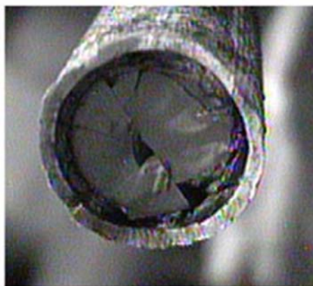
Figure 5. Cladding and bonded fuel at the rupture location after the bending test of a spent fuel pin (cladding sample cut from a BWR fuel rod with average burn up \approx 50 GWd/tU) (courtesy of AREVA TN)
