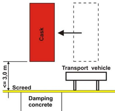
**Figure 1. Principle sketch of the considered accident scenario**
