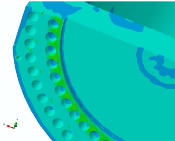
**Figure 7. Maximum principal stress (elastic/ideal-plastic closure plate -M 6-)**
