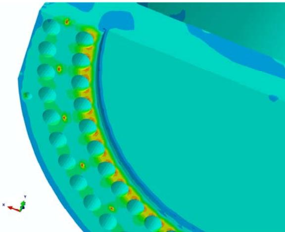
**Figure 6. Maximum principal stress (reference model -R 1-)**
