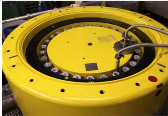
**FIG. 1 LEAK-TIGHTNESS TEST AT A PRIMARY LID**
