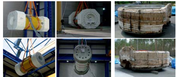
Different impact limiters designs (unequal and equal octaeder, round, round with circumferential interruptions) Impact limiter built of thin steel plates filled with wood of different kind and fiber direction
