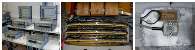
Data acquisition (left), central soldering terminal (middle), accelerometer and strain gauge on an impact limiter (right)
