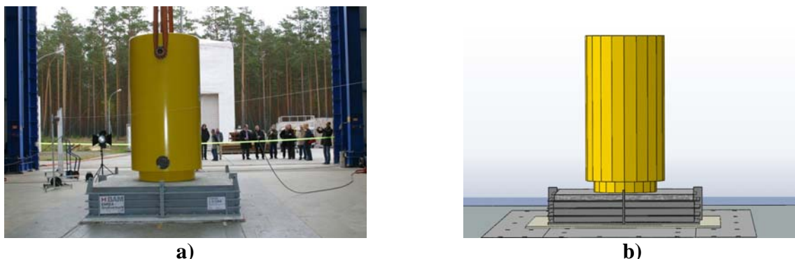
Figure 11. Drop test scenario with a cylindrical cask on top of the 500 mm thick damping concrete block
