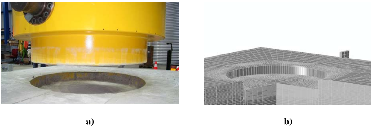
Figure 12. Imprint of the cylindrical cask into the damping concrete block after 5 meter drop test.
