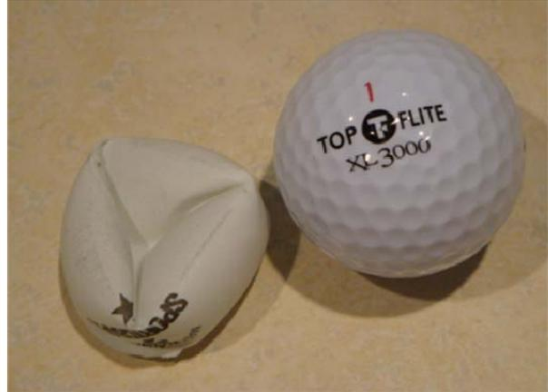
Fig. 4(b). Table tennis ball and golf ball, respectively, following the drop of a rigid weight from shoulder height onto the balls.
