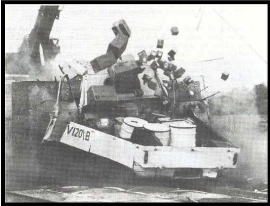
Fig. 3(a). UK impact test at 111 km/h
