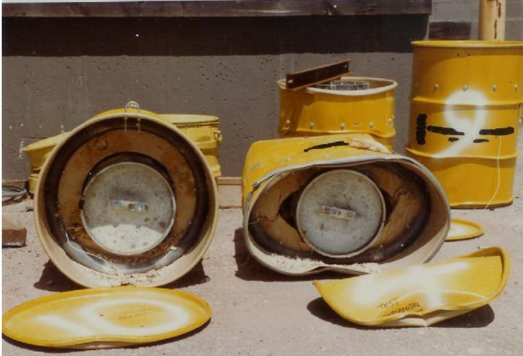
Fig. 7. Photograph of two package specimens; the package on the left was exposed to the 9 m drop test, the package on the right was exposed to the dynamic crush test (copied from Ref. 10).
