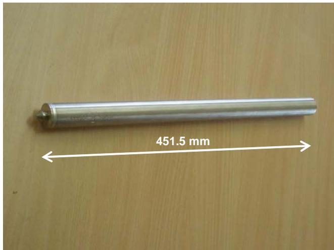
Figure 2: Source R2 for product sterilization, Manufacturer Gamma Service Recycling GmbH, Leipzig, Germany
