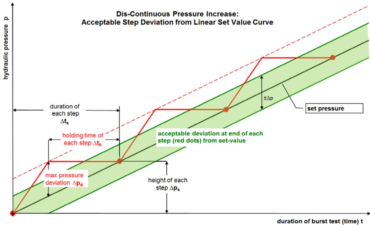
**Fig SBT-2:** *Range of pressure tolerance vs. ideal set pressure including details on stepwise pressure increase*
