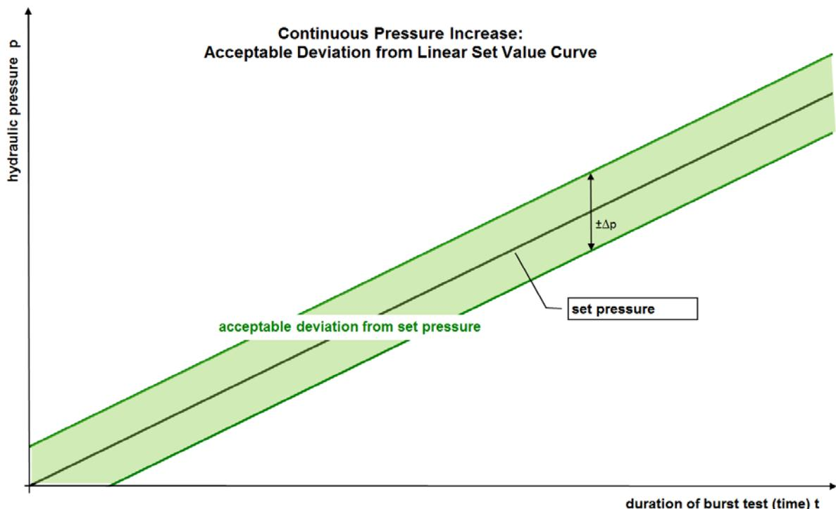
Fig SBT-1: Range of pressure tolerance related to ideal set pressure curve
